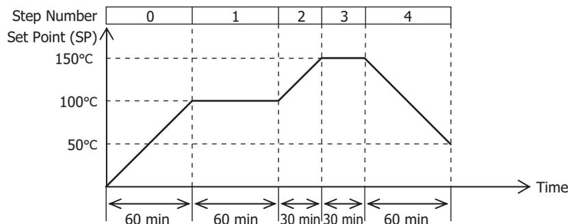
**PV Start Action [Process variable (PV) is 25°C]**
