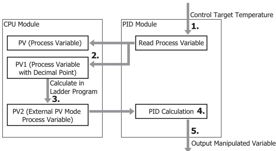
1. The PID module reads the control target temperature as the process variable.
