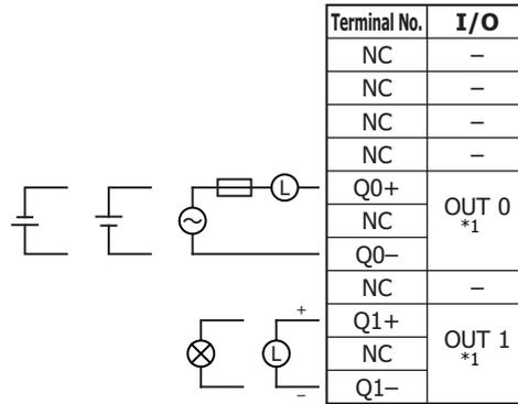
\*1 OUT0: Relay output and OUT1: Non-contact voltage/current output connection examples are shown. There are no models with both types of specifications.
