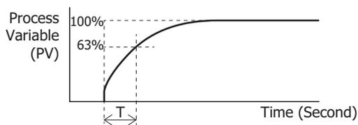
Figure 2. Process variable (PV) after PV filtering process
