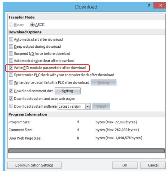
Click the check box on the left of **Write PID module parameters after download** and click **OK** button. The user program will be downloaded. After downloading the user program, the PID module parameters will be automatically written to the data registers in the CPU module and the PID module connected to the CPU module.
