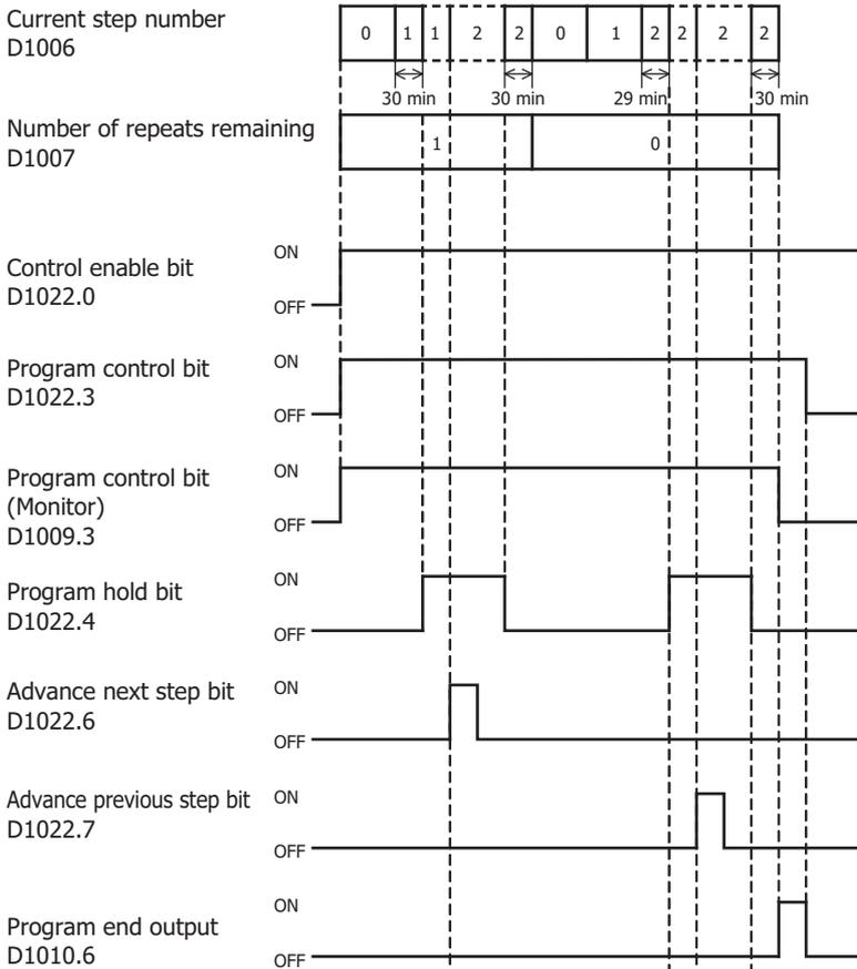
The program control is proceeded to the start of step 2 while the program hold is maintained.
