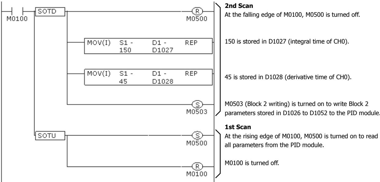
\*1 If the reading all parameters bit (M500) is turned on, all PID module parameters are read out from the PID module and stored in the data registers. Block 2 parameters are stored in D1026 to D1052.
