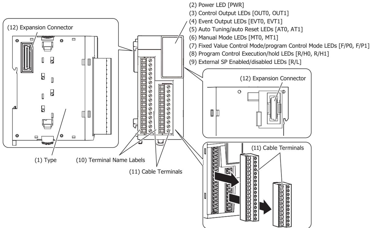
The content in brackets is the LED indicator name on the PID module.
