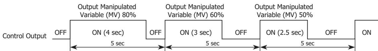
**(3) Control Register+46: Output Manipulated Variable Upper Limit**
