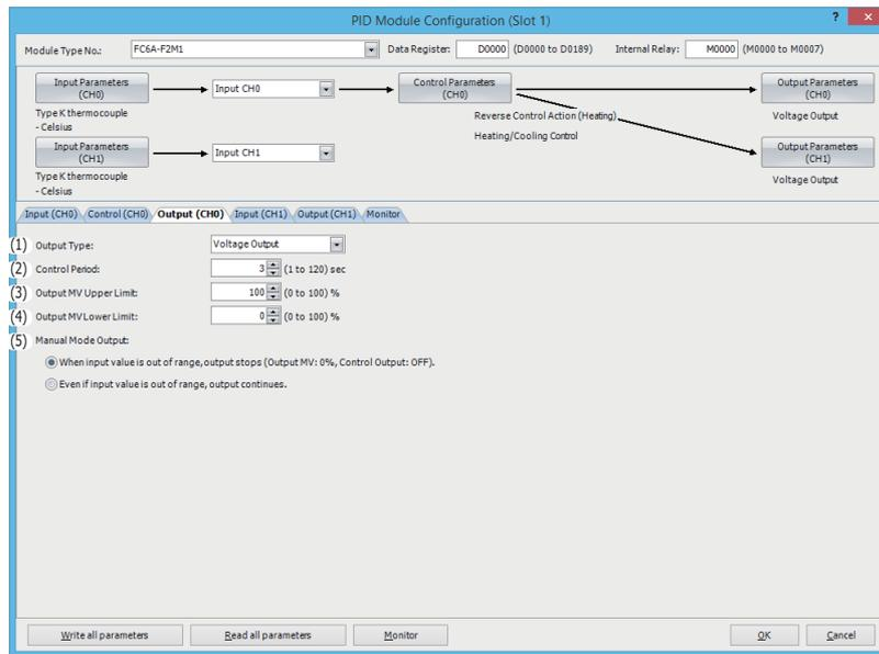
Output Parameters when Heating/Cooling Control is Enabled
