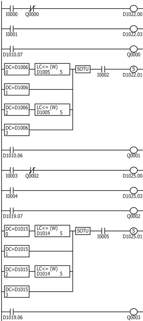
While external input I0 is on, CH0 control is enabled. When Q0 (CH0 control upper limit alarm output) is on, CH0 control is disabled.
