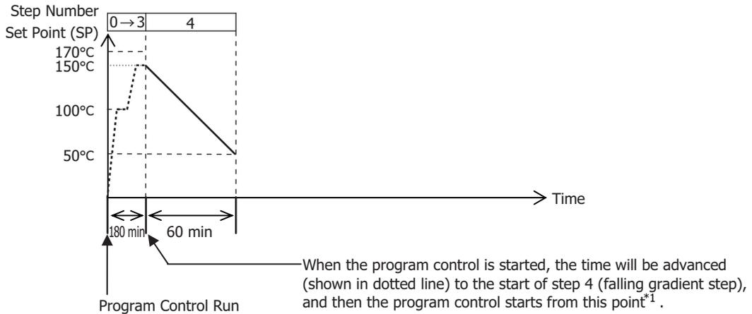
\*1 In the above program pattern, if the set point (SP) of step 4 is 0°C and the step time of step 4 is 0 minutes (falling gradient step does not exist), the time will be advanced to the end of Step 3, and the program control will be terminated.
