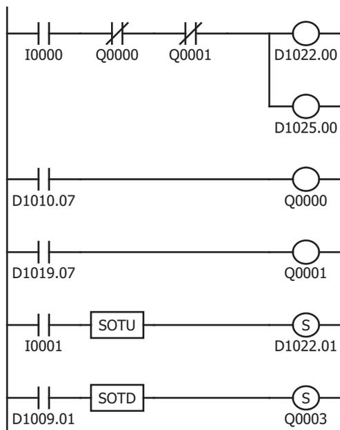
While external input I0 is on, the control of the PID module is enabled. When Q0 (CH0 control upper limit alarm output) is on or when Q1 (CH1 control upper limit alarm output) is on, the control of the PID module is disabled.
