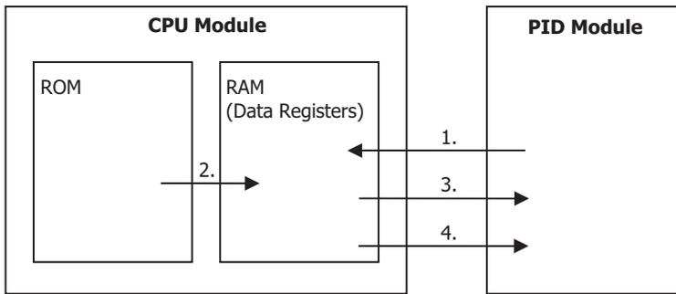
1. All parameters are read out from the PID module and stored in the data registers in the CPU module when the reading all parameters bit is turned off to on.
