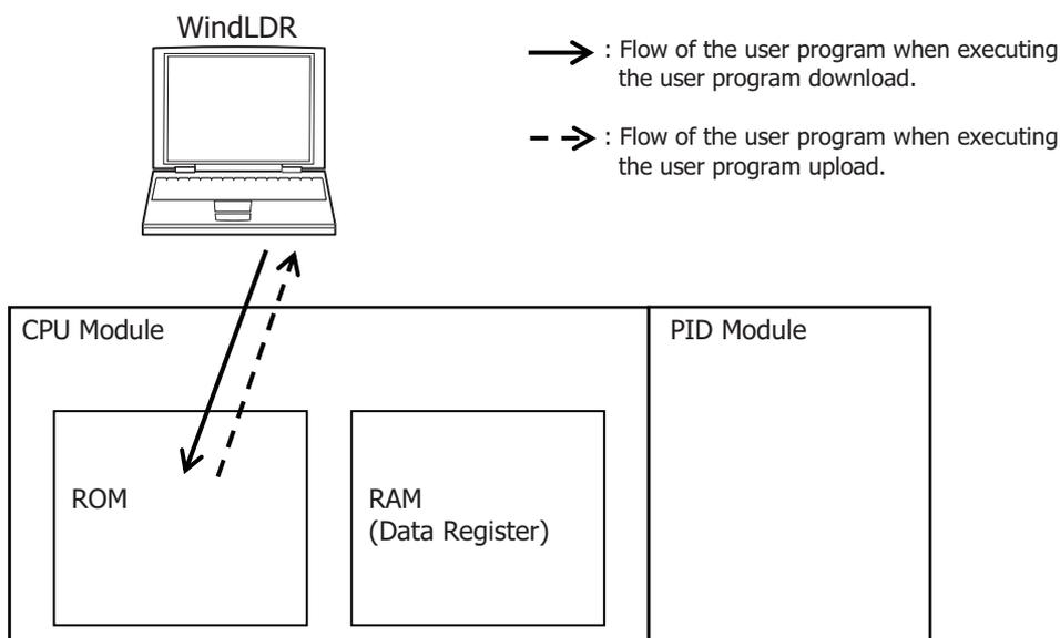
\*1 When the **Write PID module parameters after download** check box is selected in the **Download** dialog box, the parameters will be written after the user program is downloaded to the CPU module. The PID module parameters are written to the data registers in the CPU module and the PID modules with the slot numbers that were inserted with the Module Configuration Editor. For details, see "User Program Download" on page 6-4.
